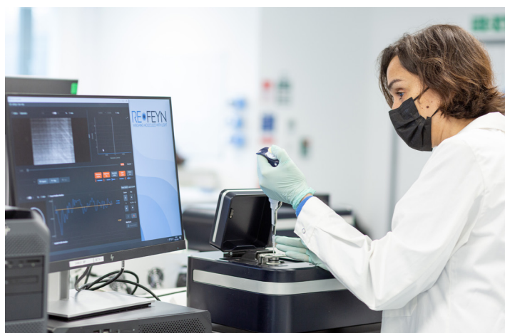
Fig. 1 The Samux MP mass photometer, a benchtop instrument. The Samux MP requires very little sample for each measurement (20 \mu L of sample diluted to 1 \times 10^{11} capsid particles/mL is optimal). Measurements are simple and can be performed in a wide range of buffers.
